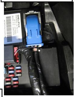
3. Remove the blue wire connector, then remove the black fuse box cover by pushing the latches away.
