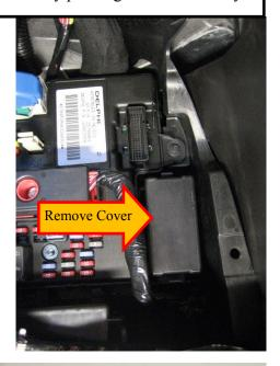
6. Inspect the Fuse Jumper. The left terminal, shown by the red arrow, MUST go to the WSW HOT socket.
