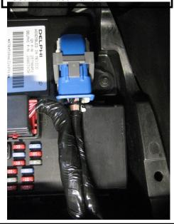
4. Remove the red 10 amp Windshield Wiper Fuse and the yellow 20 amp Power Outlet Fuse with the fuse puller.
