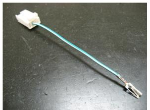
Look closely at the photos on my website at: http://www.kawal.net/navigation.htm to see how the female terminal must be removed from the 12 pin connector you pulled from the back of the Navigation unit. To remove the terminal, you must first remove the gray TPA (terminal position assurance). The TPA prevents any of the terminals from being removed. It is shown behind the blue arrow in the photo below left.
