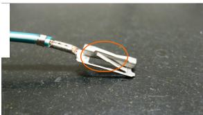
See the locking tab in the orange oval above? Use a small jewelers screwdriver to push the tab down as you gently pull on the original green/white wire in the 12 pin connector. Once you remove it, if the tab is distorted, use the screwdriver to bend it back in place so it will again lock into the new 2 pin connector.
