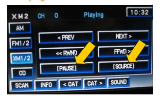
The new SOURCE button allows the user to enter two new modes of operation, DIRECT mode and AUX mode.
