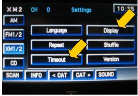
If the Timeout button is ON, the Nav screen will default to the Playing menu after 10 seconds of inactivity.
